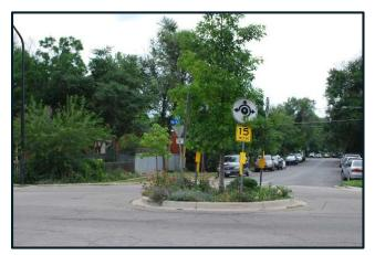
A traffic circle consists of a raised curb area installed in the middle of an intersection that requires drivers to travel around the obstruction as they enter the intersection. This is similar to the concept of a roundabout, but with a smaller footprint and slower speeds, as appropriate for neighborhood intersections.
