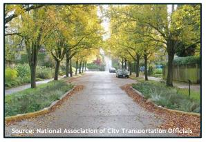
A pinch point is a series of two curbed areas on the edge of travel lanes that narrow the usable travel width to only allow for one-way traffic. This slows drivers to navigate the one-way section and also may convey the roadway is a local, slow-speed road.
